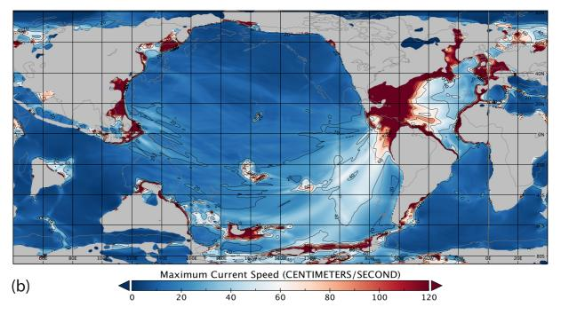
Figure 4. (a) Maximum tsunami sea surface perturbation heights and (b) maximum flow velocity at each grid cell. Contours are shown for every meter of amplitude (saturated at 1,000 cm) and every 20 cm/s of speed. Contours of modern continents are shown for reference as gray lines. The results of the MOST model are shown here, because our MOST simulation saved output more frequently than our MOM6 simulations.
