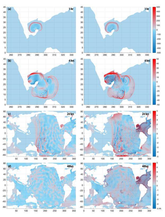
Figure 3. Comparison of two tsunami propagation models: MOST model—left column, MOM6—right column. Sea surface height perturbation in meters shown at (a) 1 hr and (b) 4 hr after impact around Gulf of Mexico, (c) 24 hr and (d) 48 hr post-handoff globally. Animations for both models are provided in Supporting Information Movies S3 and S4.
